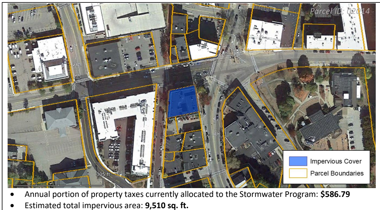
Figure 6: Example of a Downtown Commercial Property's Current Funding Contribution to the Stormwater Program
