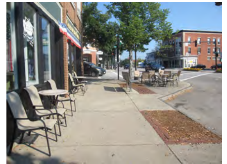
Sidewalks with street tree planter pits.
