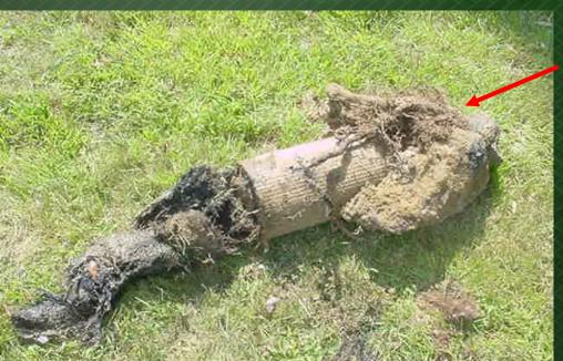
Root mass pulled from Interior of sewer line
