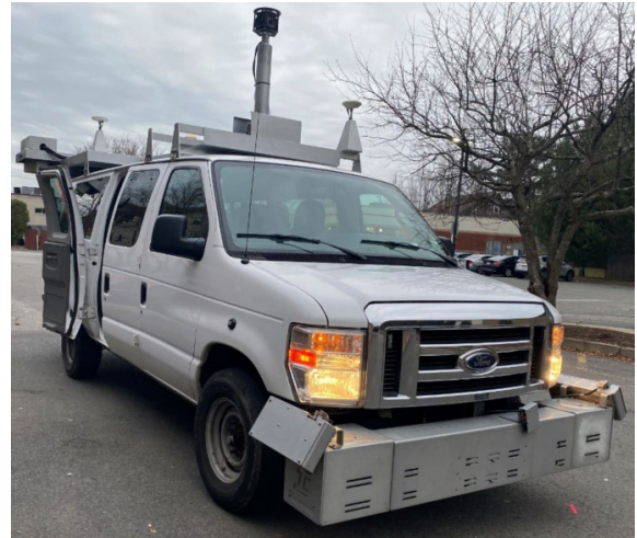
Figure 4: Stantec's Road Tester 3000 for rating paved roadways.
