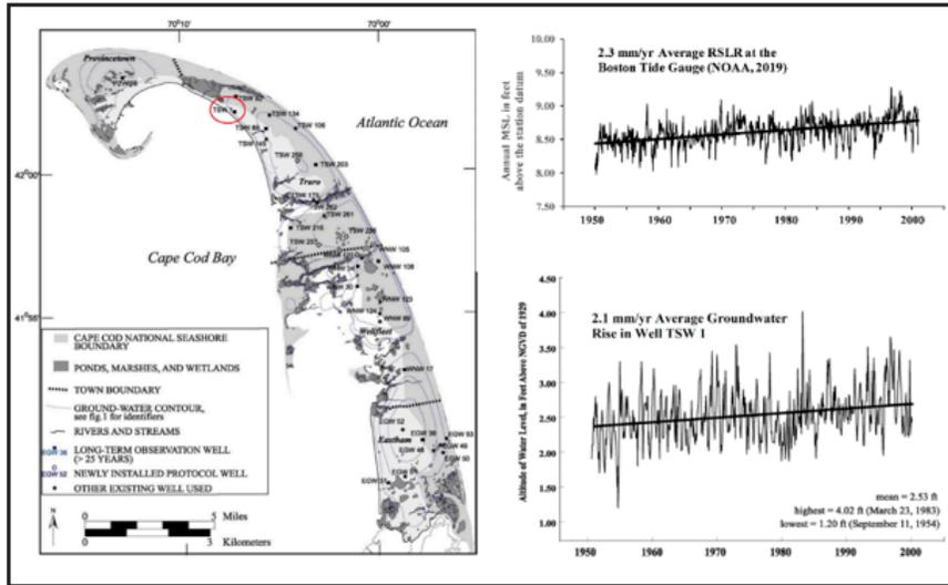
**Figure 6.2.** Groundwater levels measured in well TSW 1 compared with surface-water levels measured at the Boston tide gauge (NOAA, 2019). TSW 1 is circled in red on the map of outer Cape Cod. **Source:** McCobb and Weiskel (2003).
