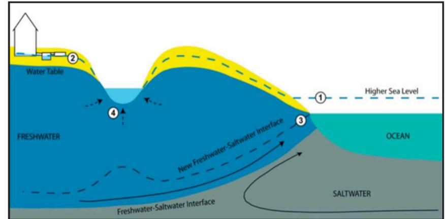
**Figure 6.1.** Schematic drawing showing the interconnected system of groundwater (fresh and saline) and surface water. Some consequences of rising groundwater are indicated: (1) SLR-induced groundwater rise, (2) septic system failure and basement flooding, (3) landward movement of the freshwater/saltwater interface, and (4) increased groundwater discharge to streams. **Source: U.S. Geological Survey; not to scale, vertically greatly exaggerated.**
