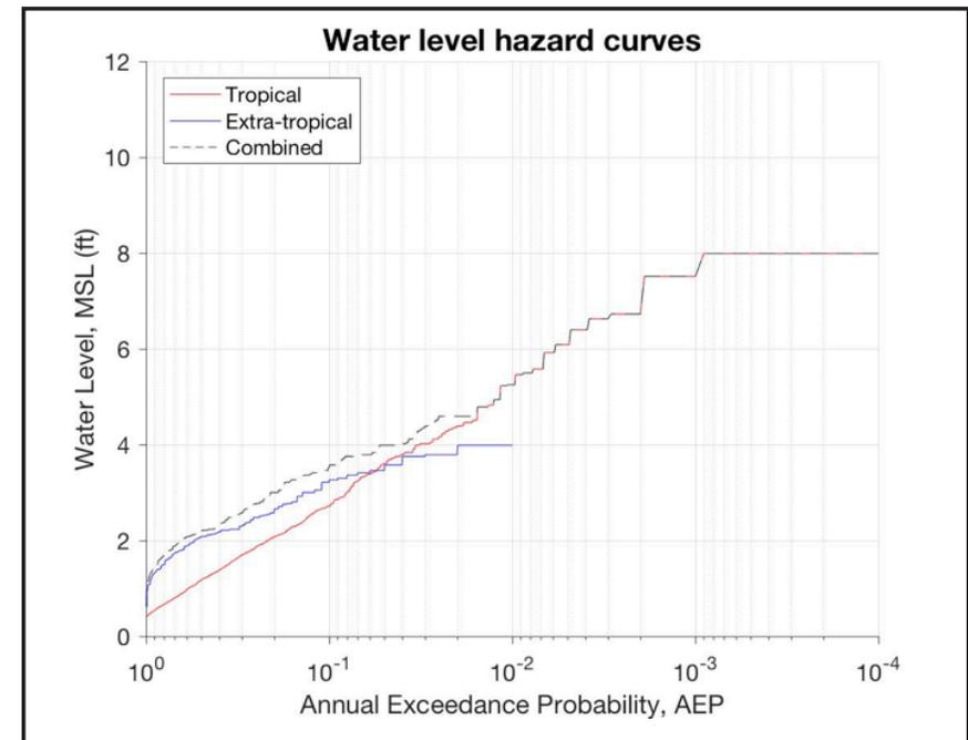
**Figure 5.1.** Water level hazard curves as a function of annual exceedance probability (AEP) for simulated tropical, extra-tropical, and combined storm distributions of surge maximum from the NACCS model save point near the mouth of the Piscataqua River in 33-foot water depth. An AEP of 0.1, 0.01, and 0.001 corresponds to the 10-, 100-, and 1000-year events, respectively. **Source:** Lippmann et al. (2019).
