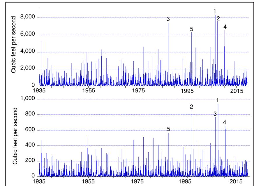
**Figure 8.3.** Daily peak discharge for the Lamprey River at USGS gage 01073500 (top) and the Oyster River USGS gage 01073000 (bottom) from 1934 through April 2019 (USGS, 2019). Note the largest five floods (ranked one through five for each record) on both rivers have occurred since 1986 (flood dates listed in Table 8.1).
