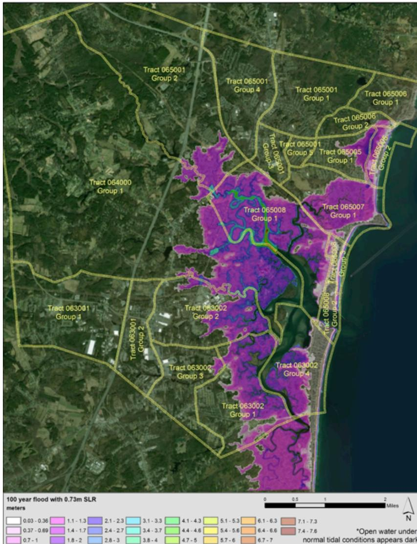
**Figure 5.2.** Inundation extent for Hampton-Seabrook Estuary under the 100-year (1%) storm surge event with relative sea level (RSL) rise of 0.73 m/2.4 feet occurring at MHW.
