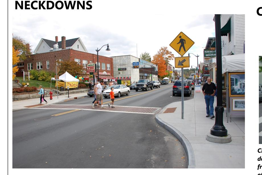
Neck downs are curb extension at midblock or intersection corners that narrow a street by extending the sidewalk or widening the planting strip and give the perception that speeds should be reduced. Neck-downs can be applied at cross walks to reduce the distances of the crossing. Typically designed to narrow road to 20 feet for two-way traffic and the drainage should be a key consideration.
