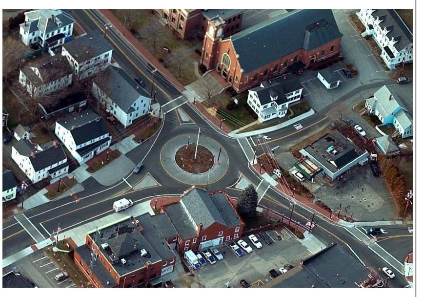
*Roundabouts are channelized intersections where traffic moves in a one-way* direction around a raised central island which is usually circular in shape. They should be fitted to the characteristics of the intersection and designed so that emergency vehicles and trucks can easily navigate the circle. A smaller version of the roundabout is the traffic circle or intersection island which are raised islands around which traffic circulates.
