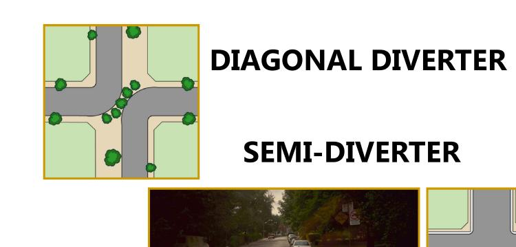
A diagonal diverter is a barrier placed diagonally across an intersection to
