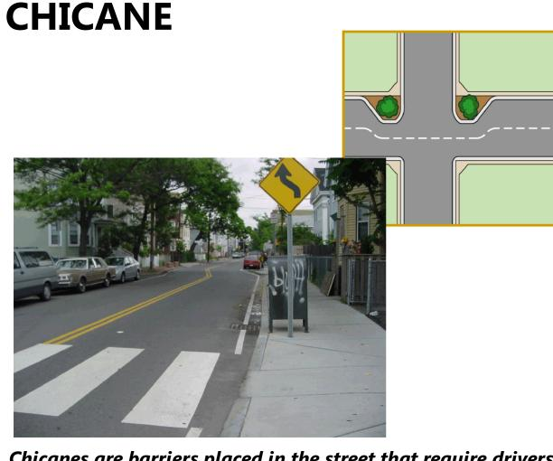
Chicanes are barriers placed in the street that require drivers to slow down and drive around them. The bulb-out sections are alternated from one side of the street to the other to create a chicane. Any type of barricade or post
