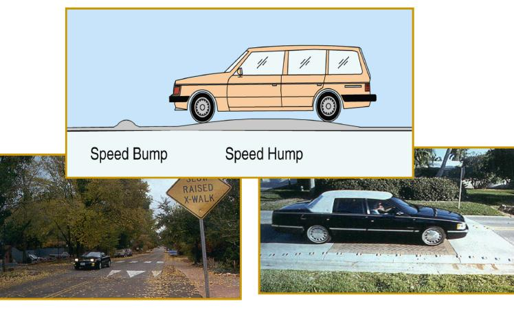
Speed humps are raised areas in the paved surface of a street that extend across the roadway. The various speed humps and speed tables can vary from rounded to flat topped. Speed humps can typically be crossed at 15 to 25 mph. Speed humps typically range in length from 12 to 14 feet although other lengths used include 10, 22 and 30 feet and generally range in height between 3 to 4 inches.
