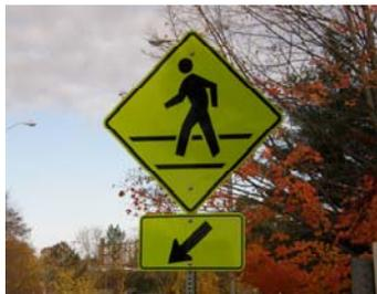
The use of any particular color scheme for pedestrian warning signs should be consistent through any particular zone or area. The mixing of standard yellow and fluorescent yellow-green within a selected site area should be avoided.
