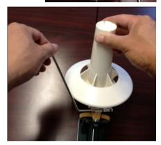
Align the bobbin and the base of the winder at the locations shown by arrows. Push the bobbin all the way down. With one hand holding the proximal wire arm to prevent the base from rotating, use the other hand to turn the bobbin clockwise to lock it down.
